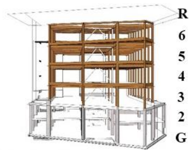
250 YEAR STRUCTURE HEAVY TIMBER, CONCRETE & STEEL
